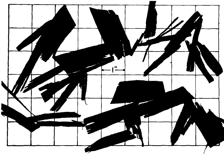
FIGURE 3 Particle geometry of disc-cut flakes produced from white oak.
